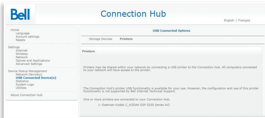
The Connection Hub's printer USB functionality is available for use. However, the configuration and use of this printer functionality is not supported by Bell Internet Technical Support.
