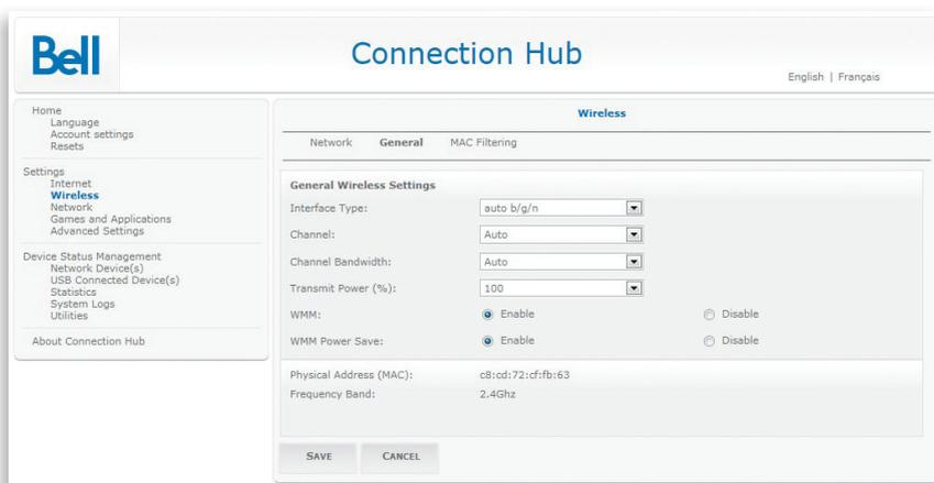
14. The **Interface type** allows you to change which wireless standard will be used when wireless clients connect with the Connection Hub. This is common for both Primary and Guest Wireless access.
